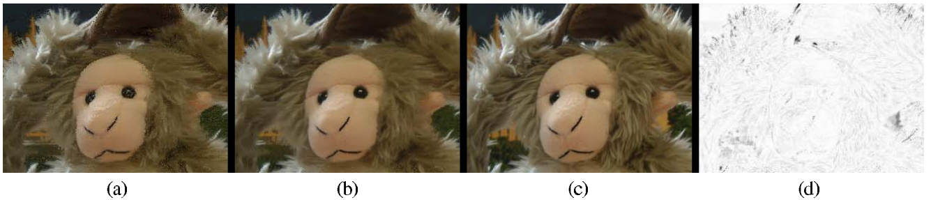
Figure 7: Leave-one-out test. Using 26 views to render a missing view allows comparison to be made between the rendered view and ground truth. (a) Maximum-likelihood view, in which each pixel is coloured according to the highest mode of the photoconsistency function. High-frequency artifacts are visible throughout the scene. (b) View synthesized using texture prior. The artifacts are significantly reduced. (c) Ground-truth view. (d) Difference image between (b) and (c).
