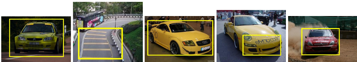
Figure 1: Example detections for the car category. From left to right the detections with the highest detection scores. The higher the score the more confident the detection.
