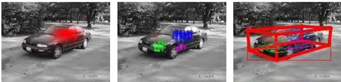
Figure 10. From left to right: a pre-detection, detected parts, initial orientation estimate, and final pose estimate.
