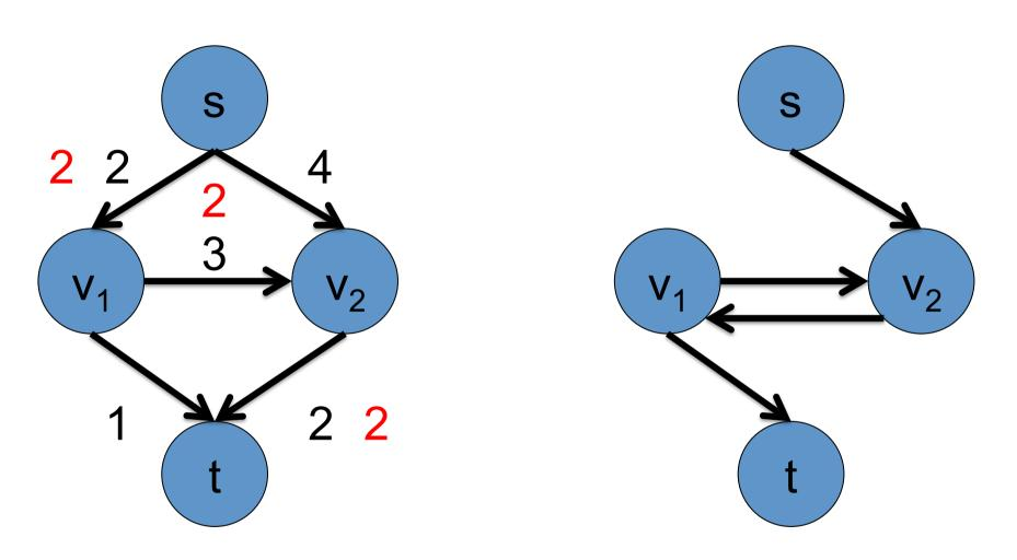
Including arcs to s and from t is not necessary Inverse of arcs where flow(a) > 0
