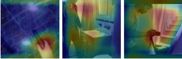
Figure 6: Conv5 activations of ActorObserverNet. The colors range from blue to red, denoting low to high activations. We observe the network attending to hands, objects, and the field of view.
