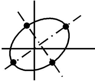
**Figure 3. The sigma points of the unscented transform.**
