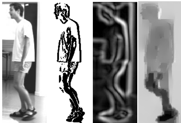
Figure 2: Image Processing Operations: original image, motion boundaries, edge detection, flow field in horizontal direction.
