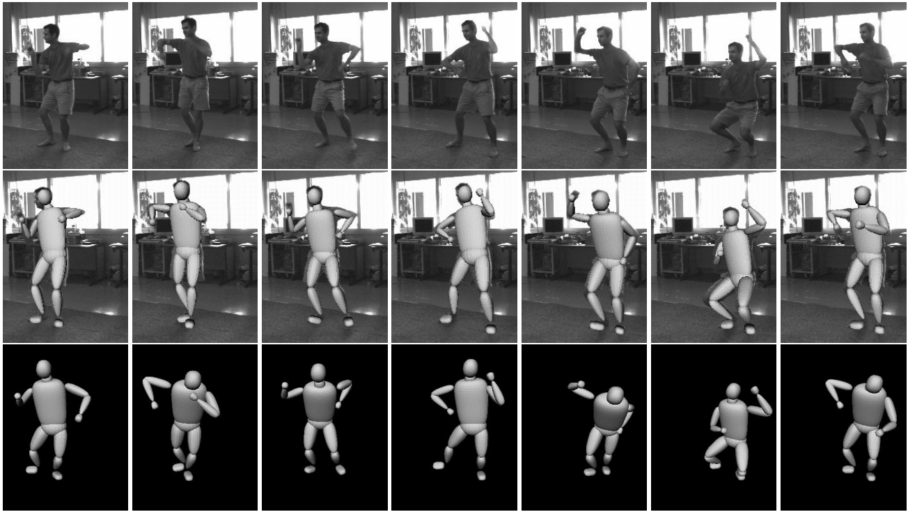
Figure 7: Jump kinematics in action! Tracking results for a 4 s agile dancing sequence. First row : original images. Middle row : 2D tracking results showing the model-image projection of the best candidate configuration at the given time step. Bottom row : the corresponding 3D model configuration rendered from above. Note the difficulty of the sequence, the good model image overlap, and the realistic quality of 3D reconstructed model poses.
