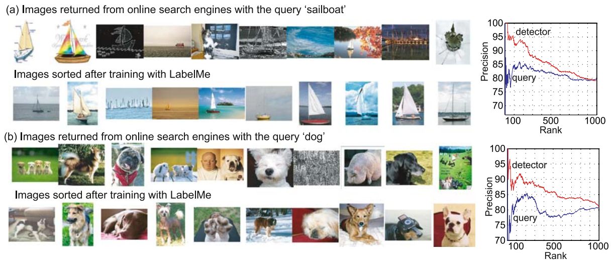
Fig. 15 Enhancing web-based image retrieval using labeled image data. Each pair of rows depict sets of sorted images for a desired object category. The first row in the pair is the ordering produced from an online image search using Google, Flickr and Altavista (the results of the three search engines are combined respecting the ranking of each image). The second row shows the images sorted according to the con-
