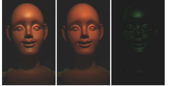
Figure 6: (a) Characteristic of diffuse pixels affected by camera noise of SONY XC-55 on head model image. (b) Input image (c) diffuse reflection component (d) specular reflection component
