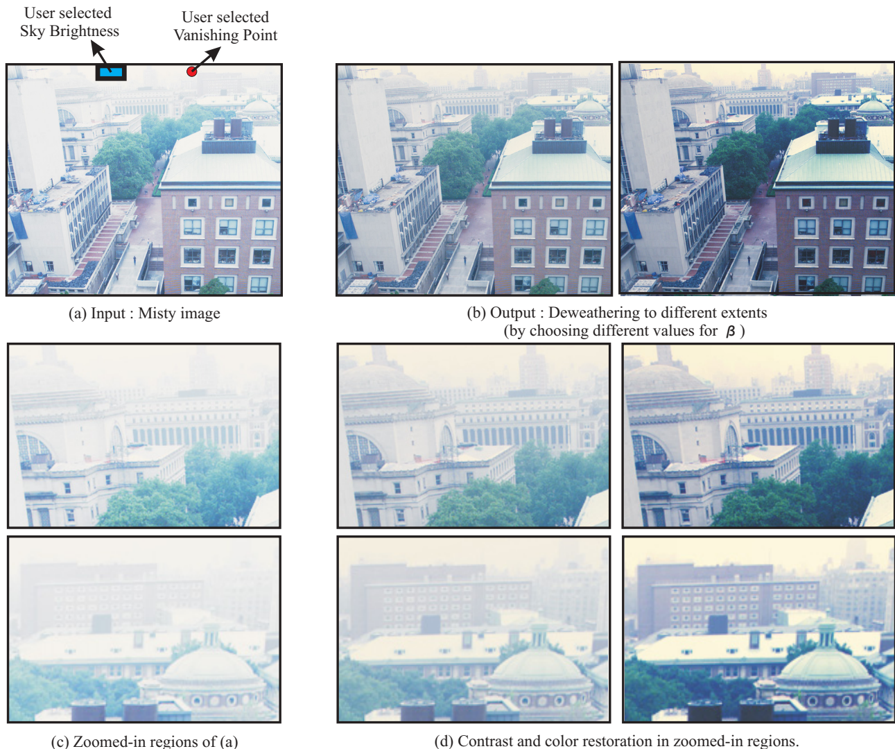
Figure 4: Restoring clear day scene colors using depth heuristics. (a) Input image captured in mist. The colors and contrasts of scene points, especially in farther regions, are corrupted severely. (b) Two images illustrating different amounts of mist removed from the image in (a). These images were computed using the depth “trend” shown in figure 3(a). (c) Zoomed in regions selected from (a) at different depths showing different amounts of mist. (d) Corresponding zoomed in regions of the deweathered images. Notice the significant color and contrast enhancement.
