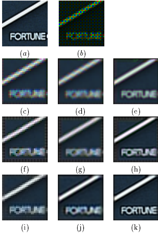
Figure 7. Reconstructed images. (a) High-resolution reference image. (b) Simulated low-resolution raw image. (c) Linear demosaicing. (d) Linear demosaicing followed by bi-linear interpolation. (e) Linear demosaicing followed by conventional super-resolution [5] (f) Demosaicing [2]. (g) Demosaicing [2] followed by bi-cubic interpolation. (h) Demosaicing [2] followed by conventional super-resolution [5] (i) Proposed, f = 1, M = 1 . (j) Proposed, f = 2, M = 1 . (k) Proposed, f = 2, M = 8 .
