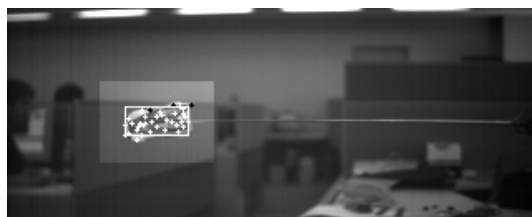
(a) High-frame-rate image with tracking result ('+' marks represent corner points being tracked. The white rectangle is a target region that circumscribes the corner points. Flicker compensation is performed in a rectangular region where brightness differs from that of other areas.)
