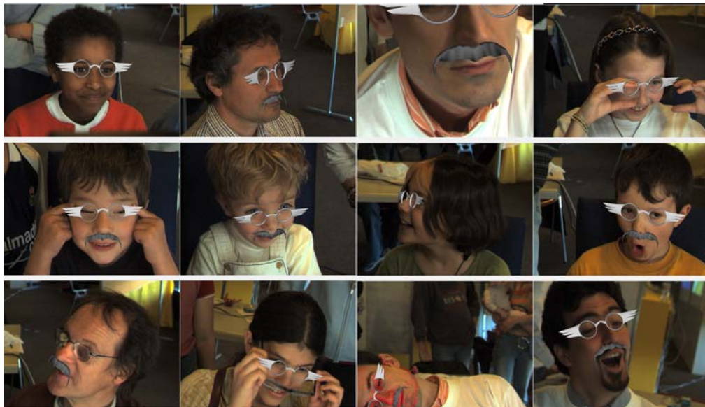
Fig.3: Screenshots from our human face tracking demo: we use a generic model to track the face of the person in front of the camera. Then, virtual glasses and moustaches are added.
