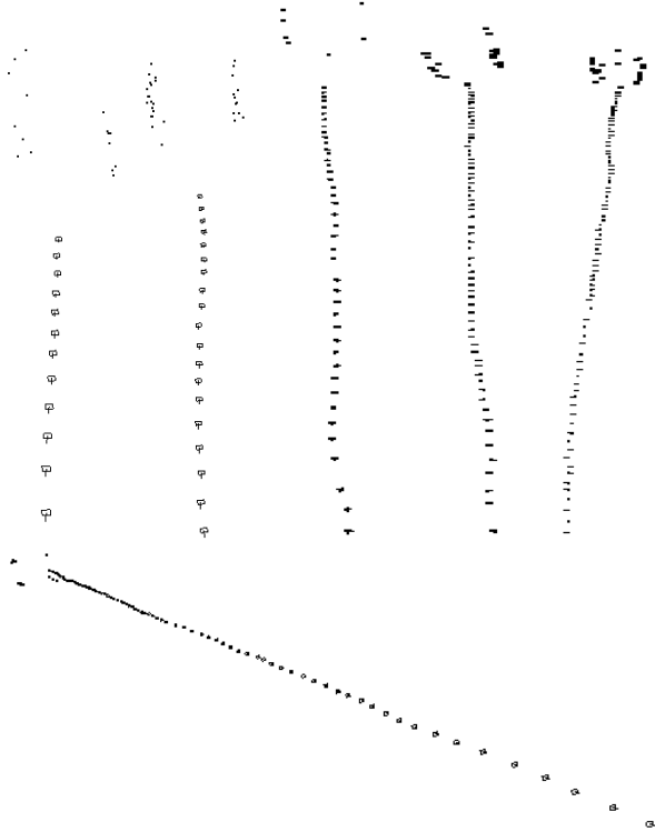
Figure 4: Estimation of the motion of a handheld camera, induced by walking down a 160 meters long corridor. The whole motion is successfully integrated into the same coordinate frame. Note how the straight trajectory builds up from left to right. The estimation was done in real-time from the tape playback. Thus, the system has to deal with capture, dropping frames if not able to keep up etc. The estimation was made with both the feature-track window and the 3D scene window displaying. In this mode, the delay from the tape to the reconstruction displaying on the screen is \sim 1 second. No prior knowledge of the motion was used and the system is identical to the one used in Figure 5.
