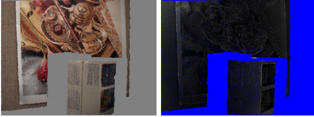
Figure 8. Prediction and absolute frame difference using correspondences estimated with LUMA.
