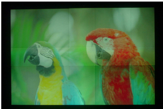
Figure 7: Result with no edge attenuation for a 2 \times 2 array of four projectors.
