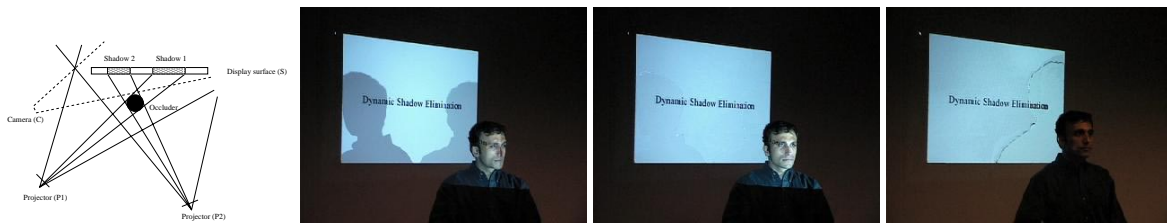
Figure 1: (a) Plan view of VRP system. (b) Passive VRP approach using “half shadows”. Active VRP approaches include (c) Shadow elimination and (d) Occluder light suppression.
