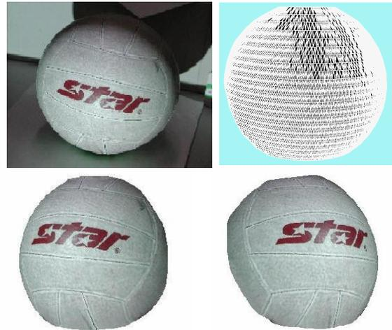
**Fig.5 The texture image of a volleyball (upper left), reconstructed 3D mesh (upper right) and the reconstruction result with texture mapping (lower two)**
